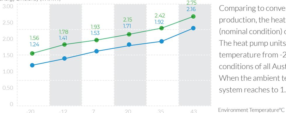
Comparing to conventional electric resistance steam production, the heat pump steam generator saves 41% (nominal condition) of electricity consumption.
